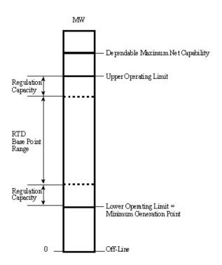
Figure 4-2 Generating Unit Operating Characteristics
