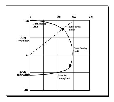
Figure 3-1 Generator MVAr versus MW Capability
